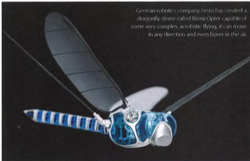
German robotics company Festo has created a dragonfly drone called BionicOpter capable of some very complex, acrobatic flying; it can move in any direction and even hover in the air.
